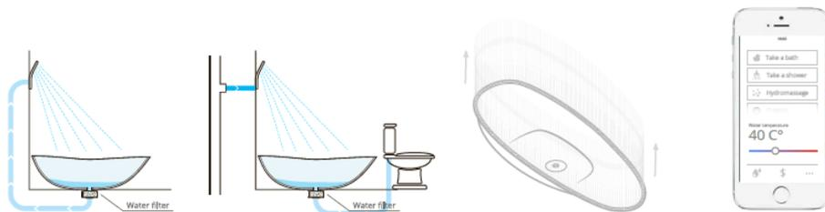
Maintain environmental care approach by introducing a looped water supply system providing stand-alone running mode;
