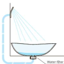
Maintain environmental care approach by introducing a looped water supply system providing stand-alone running mode;
